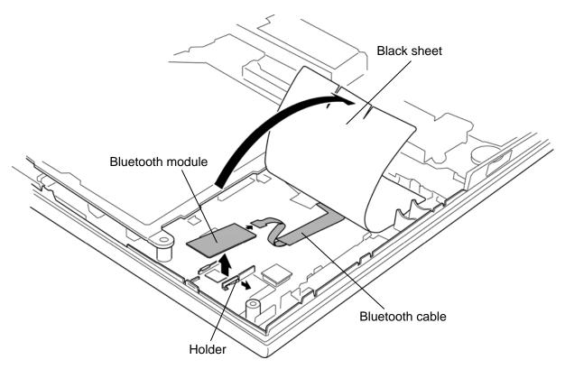
Figure 4-29 Removing the Bluetooth module
